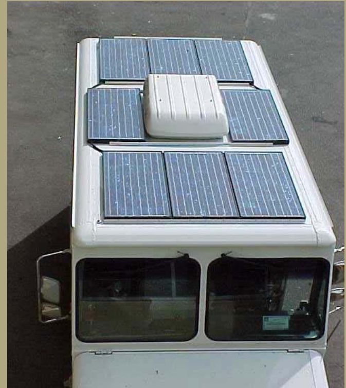
Solar panels on City maintenance vans provide mobile electricity for power tools.
