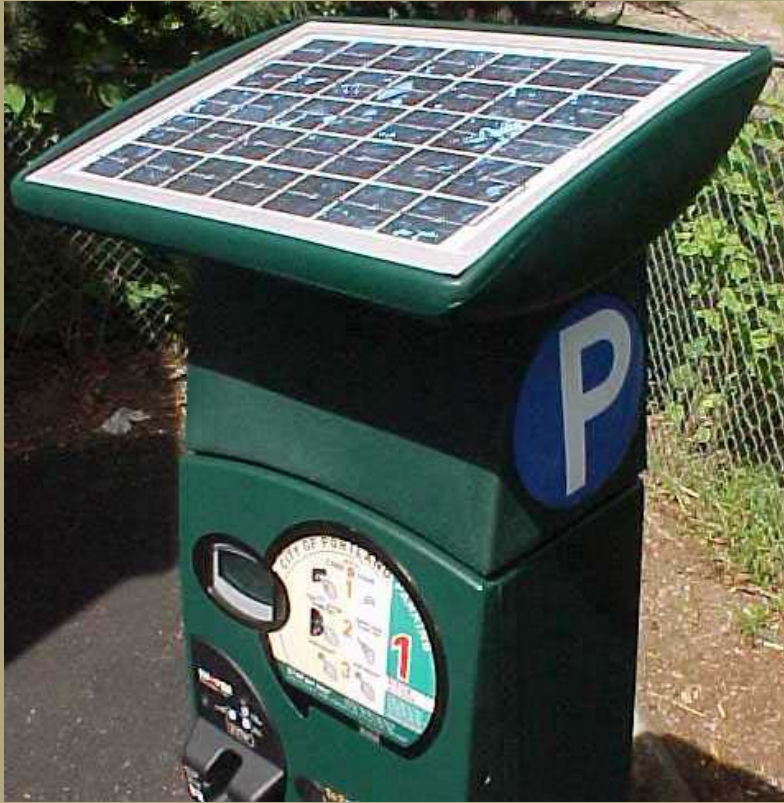
Pay stations for street parking are solar powered.
